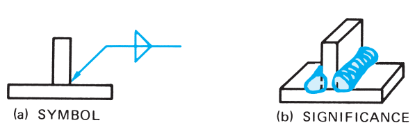
SYMBOLS AND ABBREVIATIONS Figure 30. Fillet weld, both sides.
