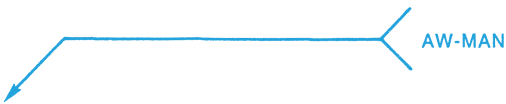
SYMBOLS AND ABBREVIATIONS Figure 50C. Suffixes indicating method of applying welding process.
