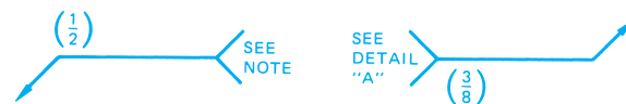
SYMBOLS AND ABBREVIATIONS Figure 46D. Size of groove weld applied to welding symbol without reference to a weld symbol.
